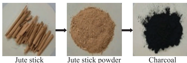
Fig 1: Preparation of charcoal from jute sticks
